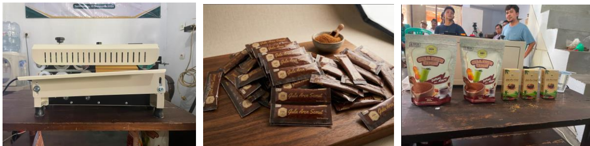
Gambar 2. (a) Mesin packing otomatis gula aren kristal, (b) Kemasan sachet-kecil gula aren kristal dan (c) kemasan dus berisi 10 sachet kecil gula aren kristal.
